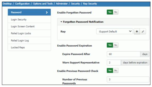
**Enable Forgotten Password** - Select Yes to include a Forgot Password link in the login dialog and send an email to a support representative with a password reset code. In the Notification field, select iSupport Default to use iSupport's default Forgotten Password notification or use the Create New and View/Edit options to access the Custom Notifications screen.
